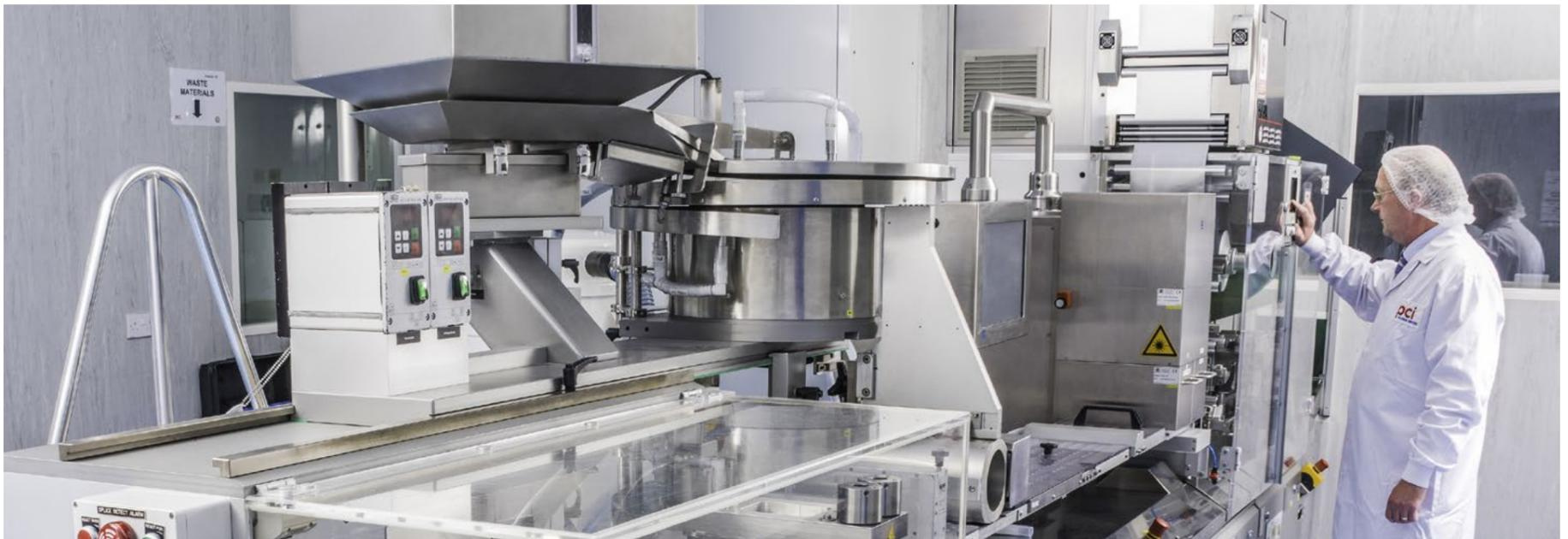
Hapa print systems are used extensively on PCI's Noack equipment. Top-mounted on the blister line, a Hapa 226 UV flexo system provides single color imaging onto foil.
