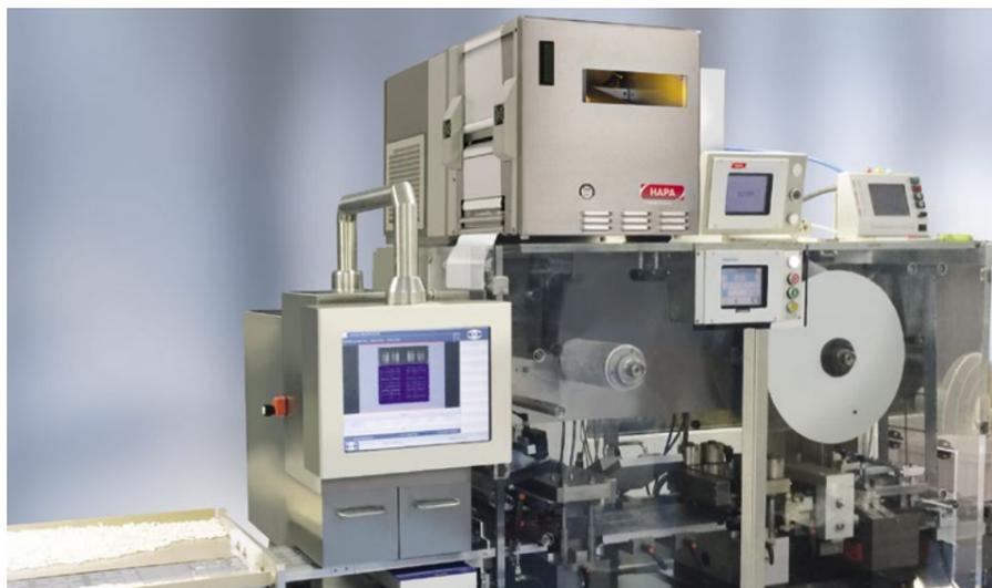
Another Hapa 226 UV flexo system working on a blister line. Inline printing is the favored approach at PCI as it simplifies the process whilst reducing waste and stock holding issues.
