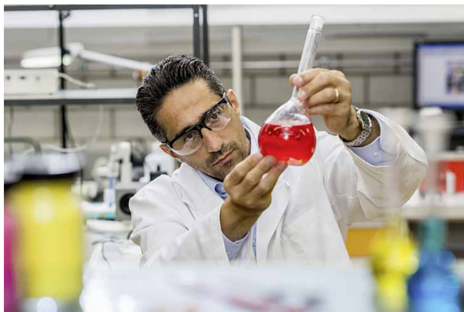
Migjen Rrahimi, Leader Ink Development, looks for the presence of small particles. Their presence may require a liquid's reformulation.
